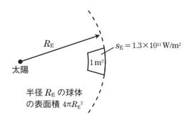
$$W_{\text{sum}} = s_{\text{E}} \times 4\pi R_{\text{E}}^2 \quad \cdots \quad 1$$
